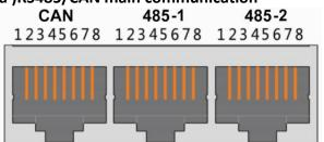
If you need to communicate with the monitoring device through RS485 or Can, the monitoring device will be used as the host, and the address setting range of other batteries will be 2~15 according to the polling data of the address.
